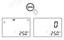
**Note:** The 0 screen will remain until a sample is measured or the instrument is turned off.
