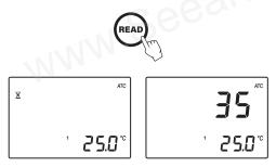
**Note:** The last measurement value will be displayed until the next sample is measured or the instrument is turned off. Temperature will be continuously updated.
